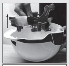
**STEP 4:** Remove the slip ratchet harness from the helmets shell.
